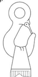
Figure D1 inadequate accommodation of a webbing eye on a hook of too small radius
