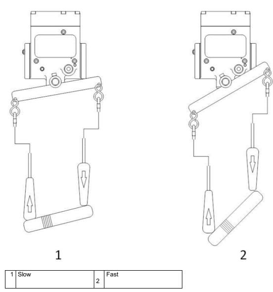
Pendant Control: the speed is proportional to the movement of the lever.
