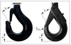
Fig. 59: Measuring hook wear
