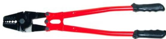
Hand swaging tool is suitable for small, soft metal and oval-shaped ferrules 2-5 mm used with steel wire ropes. The tool can be used to compress the ferrule and lock the wire rope in place, e.g. when creating a terminal loop. In addition, the tool have integrated wire cutters on the side of the jaw mechanism. Rubber coating on the handles ensures a firmer grip on the tool.
