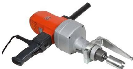
The EM 5000 power tool is very effective alternatives to manual power. Moving heavy loads will go three times faster than manually operating the winch. The EM5000 power tool has an electrical motor 230V - 50 Hz. The power tools are an alternative to the manual drive on the Holmatro WW winches and are only used for short and non-frequent applications. The combination of a hand winch and these power tools are not an alternative to an electric winch.
