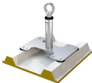
Stainless steel anchor point ABS-Lock X-SW (Ø 16 mm) with base plate (372 x 200 mm) is a fall protection solution developed for usage on top of a sandwich roof on trapezoidal sheeting (negative). To install this anchor, all you need is a minimum sandwich profile (steel) depth of 0.5 mm.
