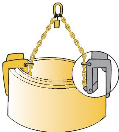
We manufacture two standard sizes of well-ring lifters for lifting and handling of concrete well rings. These have a grab width of 60–120 mm and 100–200 mm, respectively, which cater for the standard well sizes that exist on the market. High friction teeth helps to prevent sliding on ice or mud. Both sizes are available with two or three grabs.
