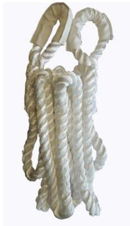
Very strong synthetic fibre rope with excellent shock absorption properties. High elongation makes this rope ideal for towing and mooring applications. Elongation: 26%. Elastic rope with loops on both ends.
