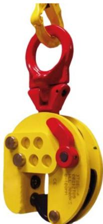
For lifting and transporting of steel plates and structures from all positions (horizontal, vertical and sidelong). Articulated lifting shackle. Jaw opening from 0 - 95 mm. Adjustable by steps of 30 mm.
